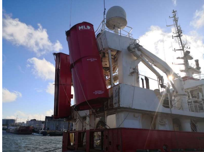
Figur 128. Multi-purpose door - MLD Trawl steering system
